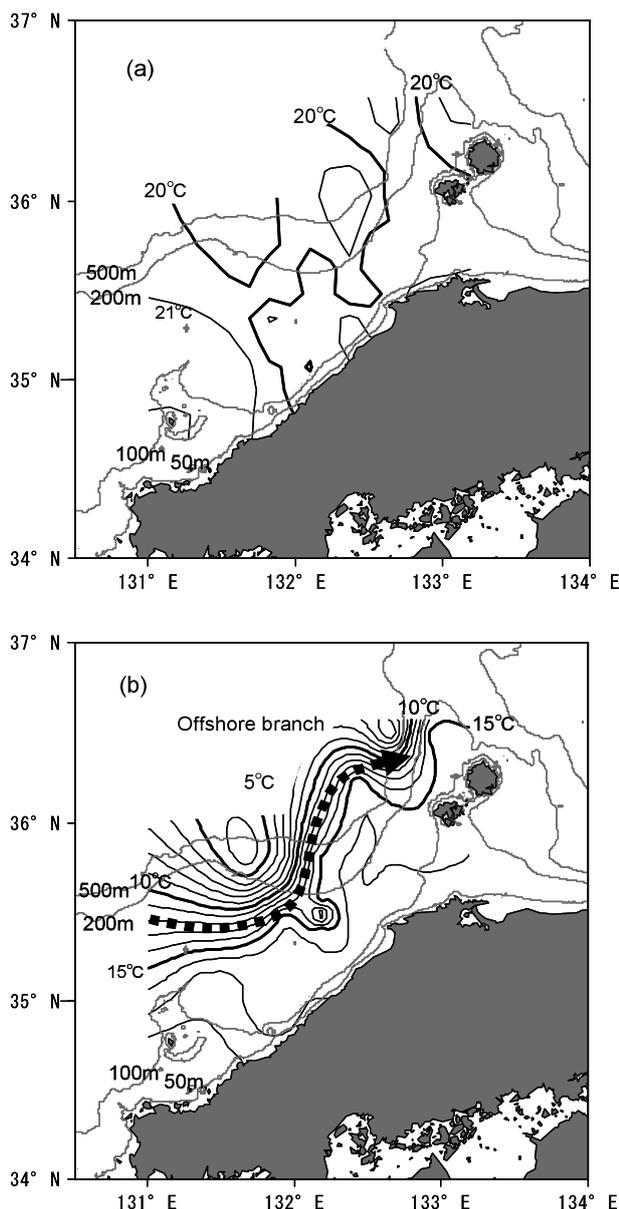
Fig.5. Isotherms at the sea surface (a) and 100m depth (b) during late May-mid July 2002 in survey area. The offshore branch of Tsushima Current was determined to flow along frontal zone in the survey area
