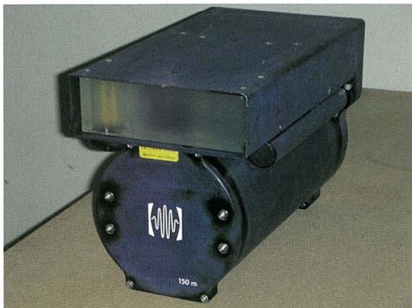
Fig. 37. Acoustic camera "DIDSON".
