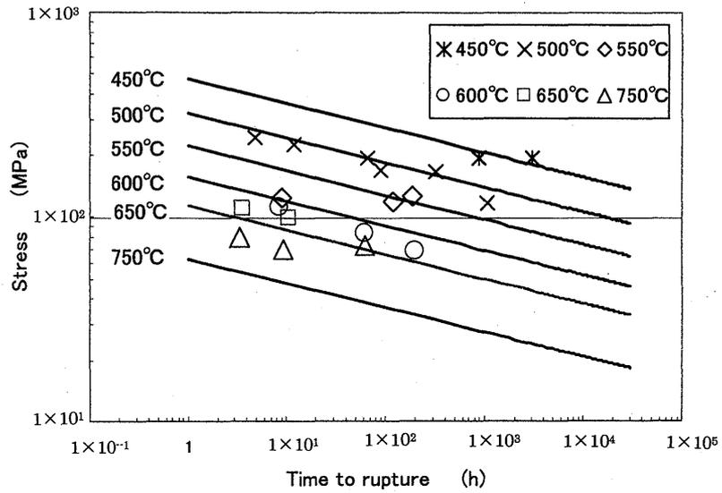
Fig. 8. Master creep curve<sup>(4)</sup>
