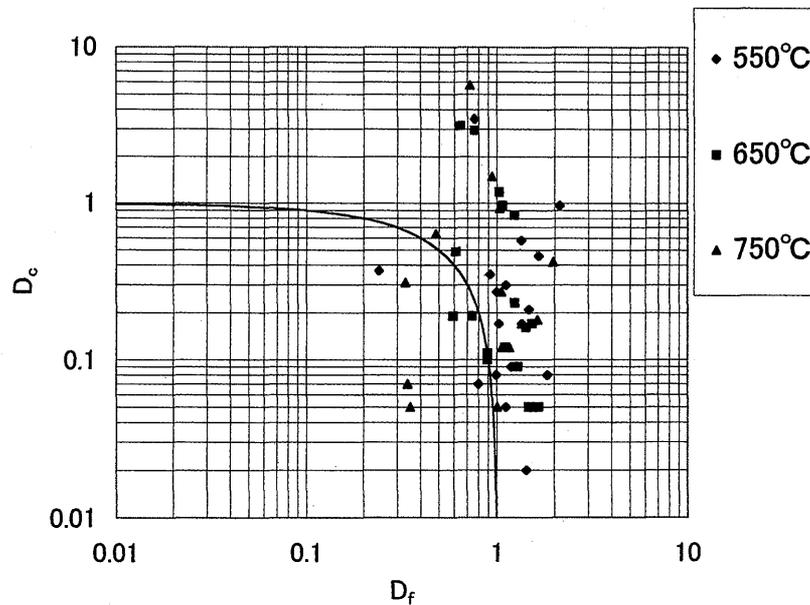
Fig. 9. Plot of creep and fatigue damages
