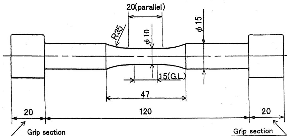
Fig.1. Test specimen configuration (unit : mm)
