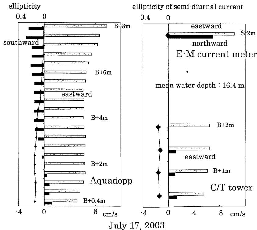
Fig. 8. Vertical profiles of the east-west (thin bar) and the north-south (thick bar) components of diurnal averaged residual currents on July 17. The marks  $\blacklozenge$  indicate the ellipticity (the ratio of the minor to the major components) of M2 constituent. The left shows those obtained from Aquadopp and the right those from an electro-magnetic current meter and C/T tower.
