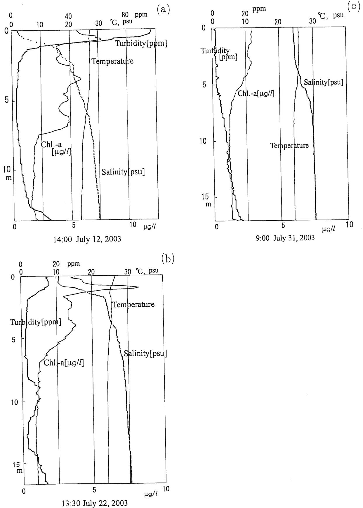
Fig. 5. Vertical profiles of water temperature, salinity, turbidity and chlorophyll-a at the mooring station. (a), (b) and (c) are those at 14 o'clock on July 12, 13:30 on July 22 and 9:00 on July 31, respectively.
