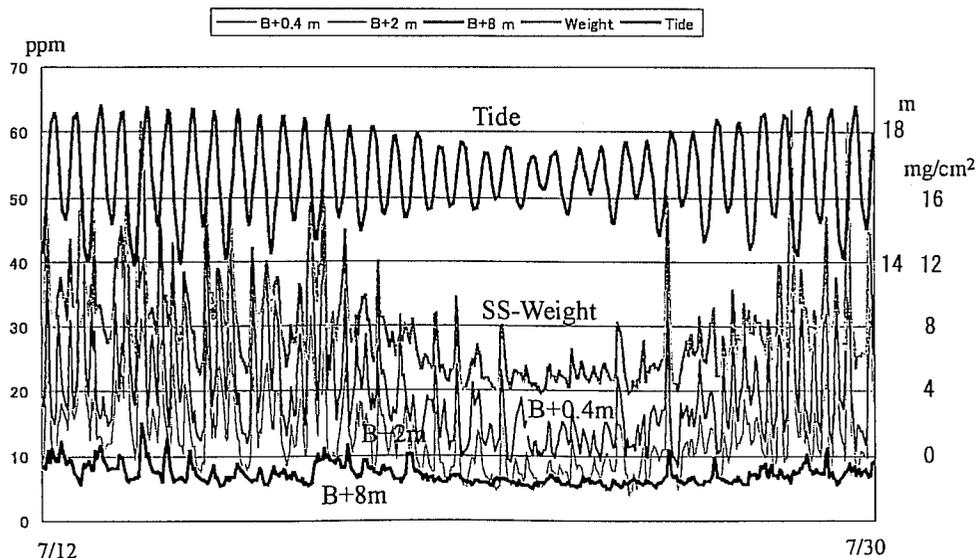
Fig. 7. Variations with time of turbidity at the levels, 0.4 m, 2 m and 8 m above the floor and the weight(mg/cm<sup>2</sup>) of suspended particles, measured by Aquadopp.
