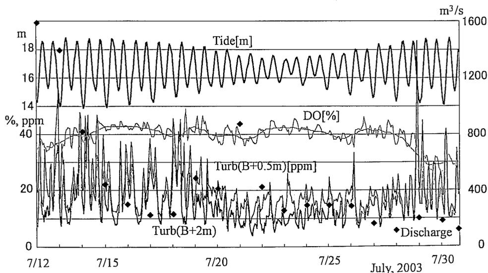
Fig. 2. Variations with time of tidal level [m], DO [%] (B+2 m) and turbidity [ppm] (B+0.5 m, B+2 m) in the duration of this experiment. The mark ◆ indicates daily averaged discharge of Chikugo river [m<sup>3</sup>/s].
