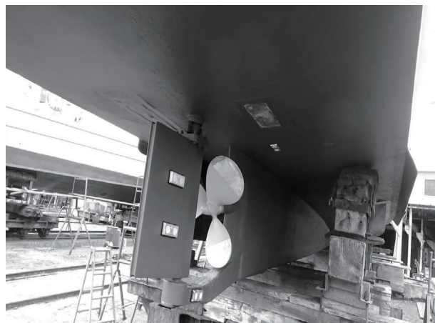
Photo3-2 Condition of rudder and propeller after cleaning
