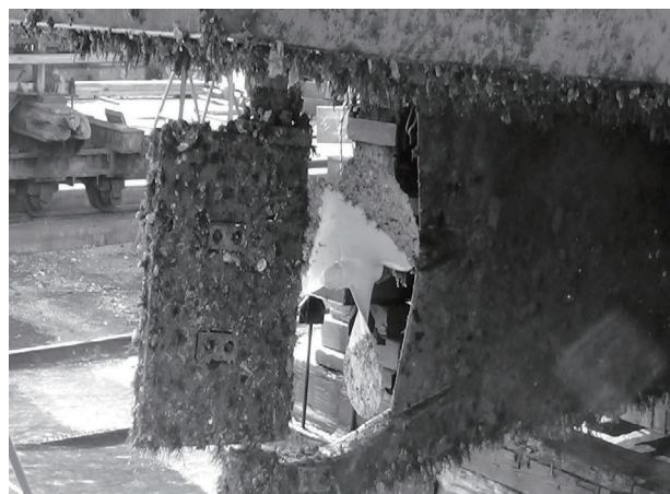
Photo2-2 Condition of rudder and propeller before cleaning
