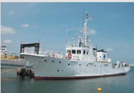
Taka-maru (Fisheries Research Vessel) Gross tonnage: 61 tons Max. passenger load: 15 persons
